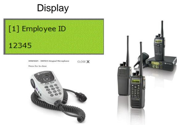
Custom FORMS can be generated using Tallysman's Windows based FORMS Builder application and loaded into the MOTOTRBO™ radio. The TW255 also supports Job Ticket dispatch with associated FORM's for Reply, e.g. Accept Job, Decline Job.
